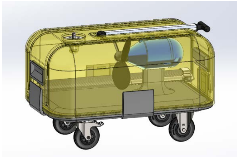
Figure 8. Hydro turbine unit in its transportation setup. The case has been made transparent for the purpose of seeing the components within the casing.
