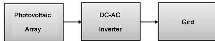
Figure 12. The topology of a grid-connected inverter.
