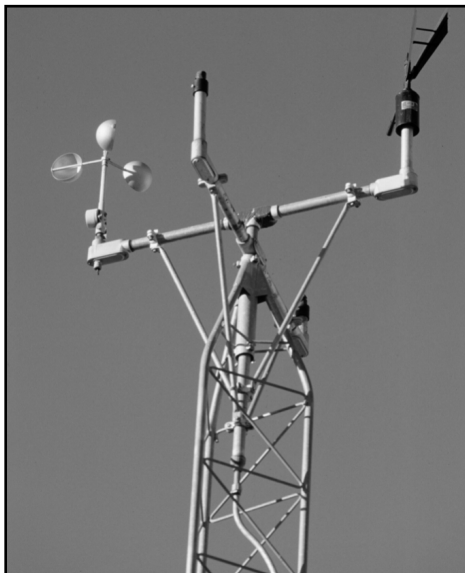
Figure 1. Anemometric tower with a cup anemometer and vane.
