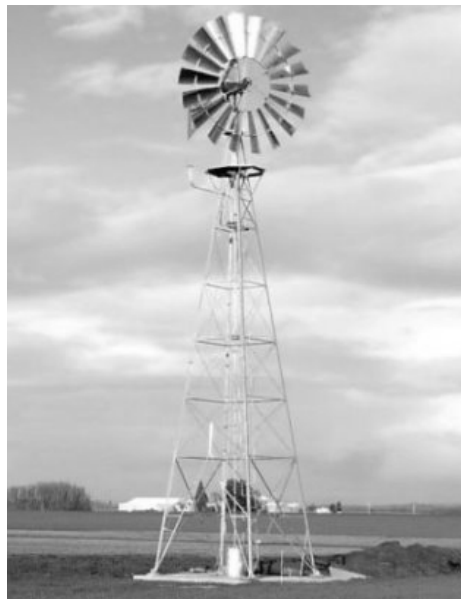
Figure 11. American windmill pump of 2 m in diameter.
