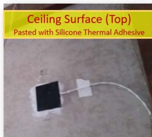
Figure 4. Photograph of HFT and a diagram showing location of heat flux transducer.
