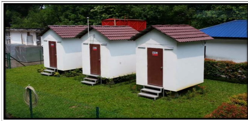
Figure 3. Three identical test huts for comparative studies of heat flow with radiant barriers.
