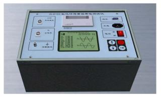
Figure 5. The virtual AI-6103 zinc oxide arrester tester.
