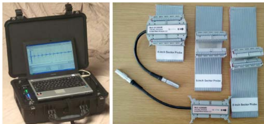
Figure 10. MsSR3030R equipment and MsS plate probe used for inspecting mockups.
