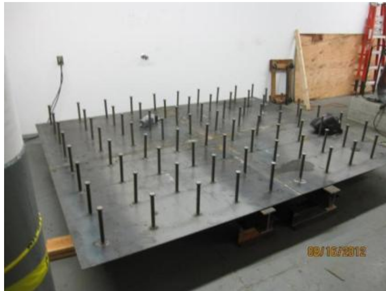
Figure 5. The straight wall PWR mock-up, “A”, lying with its OD side sticking up following welding of the four quadrants.
