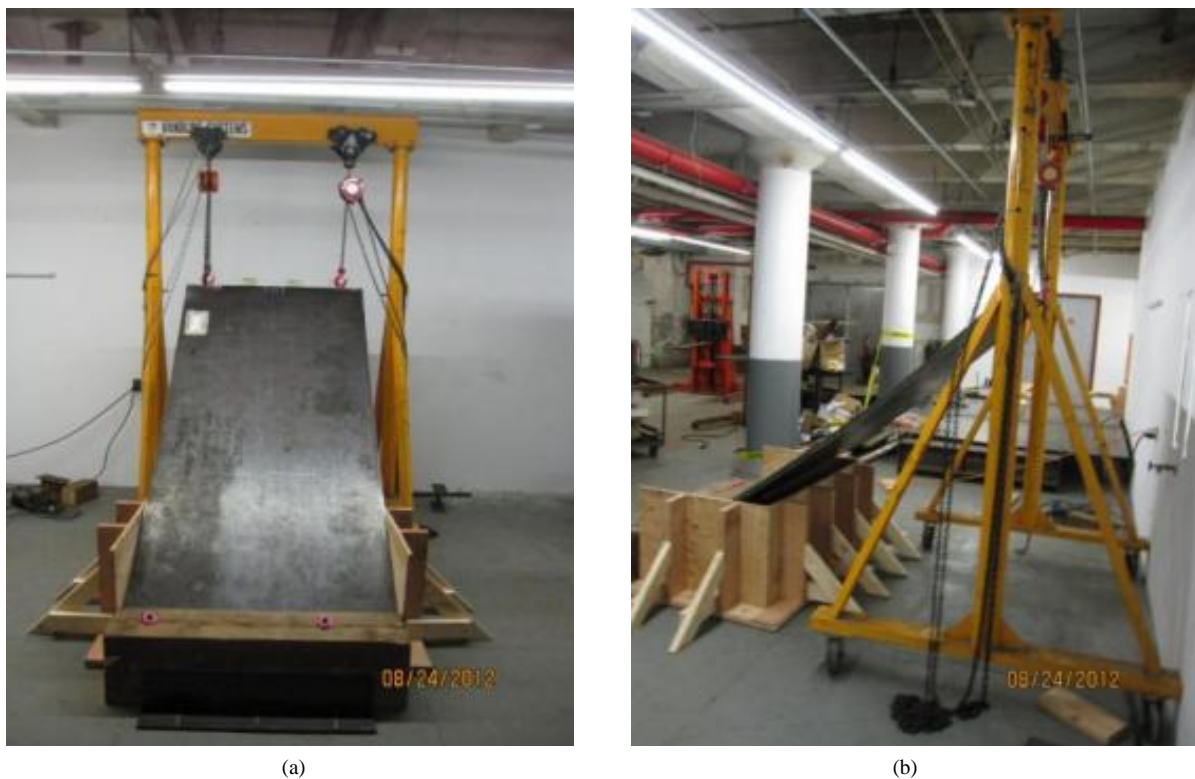
Figure 4. (a) Front and (b) side view of the BWR mock-up prior to concrete placement.
