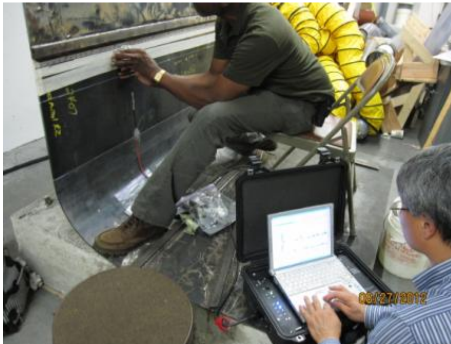
Figure 12. Baseline data acquisition of “G” mockup with MsS instrumentation.
