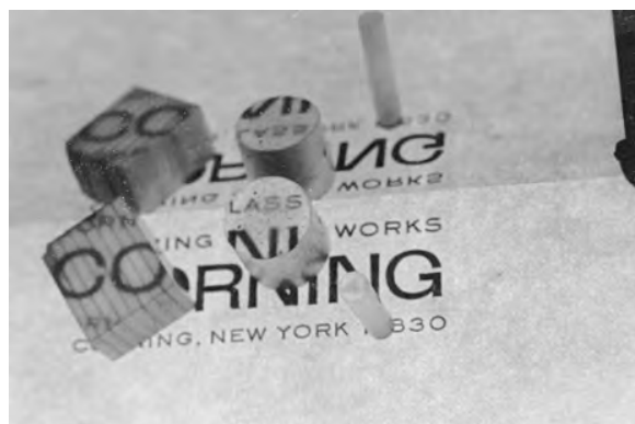
Figure 5. Example of image transfer from a much larger diameter bulk sample.
