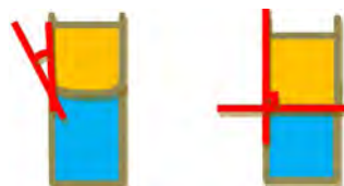
Figure 3. Variation of the contact angle of the lipophilic phase before (16°) and after (90°) addition of the surfactant [8].
