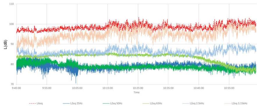
Figure 16. Examples of occurrence of Case C. The increase of sound pressure levels at high frequencies is very smooth.
