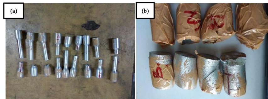
Figure 8. (a) Tensile test samples after failure; (b) Compression test samples after failure.
