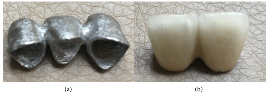
Figure 14. Laser fusion printed titanium teeth crown.
