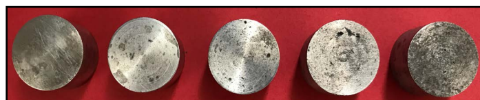
Figure 2. Samples after salt spray corrosion test.
