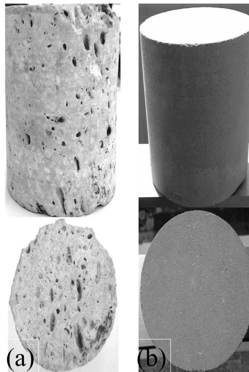
Figure 1. (a) The core has vuggy porosity which can be seen from surface and size; (b) The core has no vuggs like the other.
