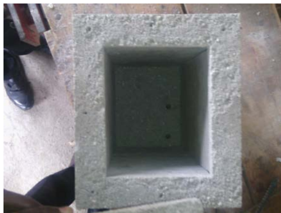
Figure 1. Picture of the setting of the refractory bricks after baking.
