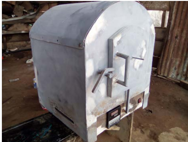
Figure 3. Picture of the oven-furnace under construction.
