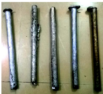
Figure 2. Al-Ni specimens having compositions of 0%, 10%, 20%, 30% and 40% nickel from left to right respectively.
