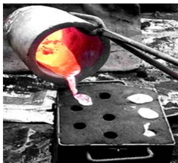
Figure 1. Sand casting being done to prepare the specimens.
