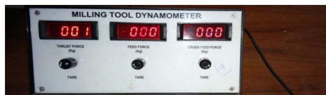
Figure 4. Milling tool dynamometer for measuring cutting forces.
