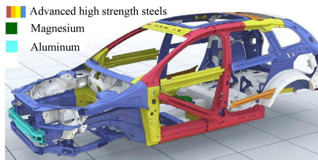
Figure 6. A schematic of Volvo-2009 model, showing the different class of materials used for designing the car body [45].
