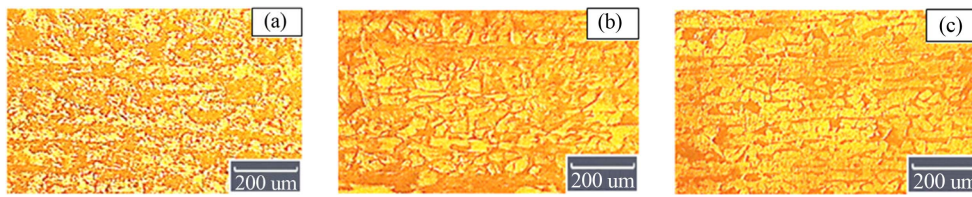
Figure 7. Photomicrograph showing the microstructure of the HAZ: (a) LHI (b) MHI and (c) HHI.
