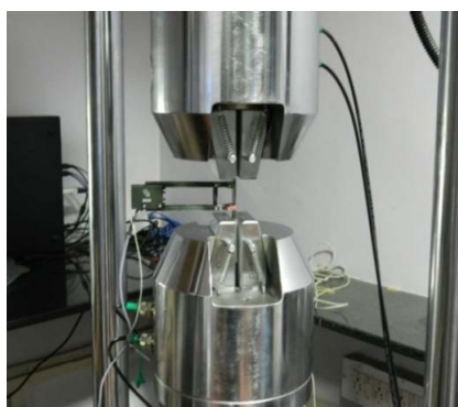
Figure 4. Specimen loaded in testing machine.
