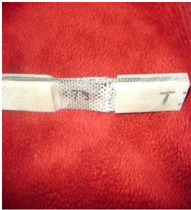
Figure 6. Failure of tensile specimen.
