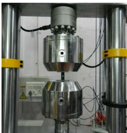
Figure 5. Specimen loaded in universal testing machine.
