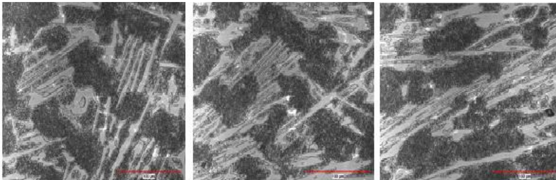
Plate 4. Annealed \varnothing 100mm bar
