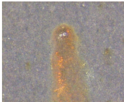
Fig. 7 Optical micrograph of WC-12Ni coating after 114 hours exposure to the salt spray test
