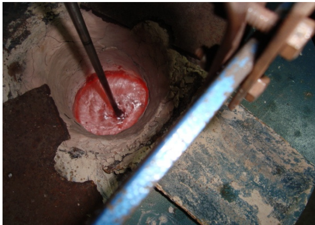
Fig.2. Stirring of liquid metal with preheated SiCp.
