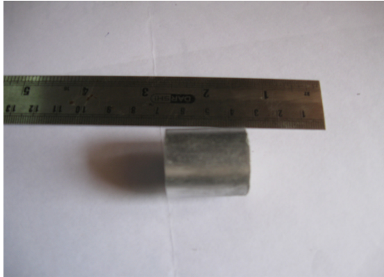
Figure 2. Cylindrical Specimen after compaction. Figure 3. Specimen c/s after extrusion.
