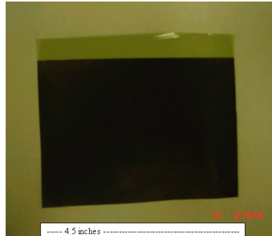
Figure 3. Picture of a dry coating of 1:1 wt/wt HiPco/VA-AA copolymer onto a Teflon™ film, which was found to have a surface resistivity of 3.5 k-Ohms/sq
