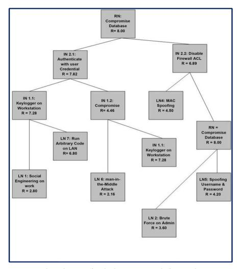
**Figure 6.** Attack tree diagrams a for school computer network after upgrade.
