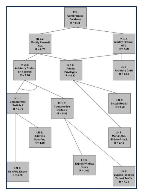
Figure 3. Attack tree diagram b for the school computer network.
