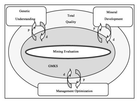
**Figure 6.** The keys to the success of mining valuation process: integration of a *Geologic and Mining Knowledge System* (*GMKS*). d: data and interpretations; p: processing results and synthetic information.
