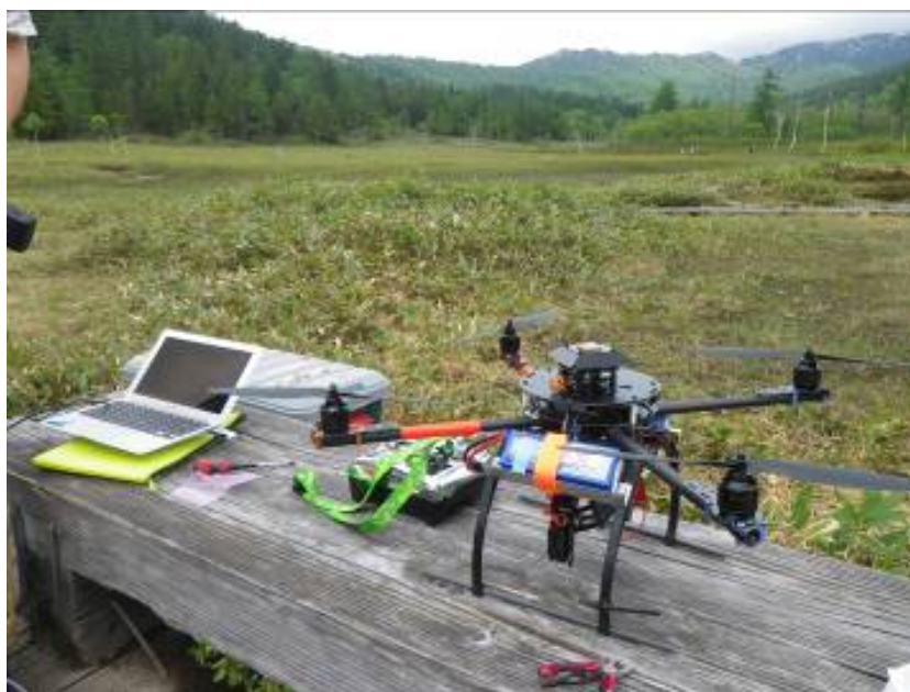
Figure 2. UAV (unmanned aerial vehicle) system. *Radio-controlled helicopter used in the study (MK EASY Okto XL2 1.5 CFK Edition of HiSystems GmbH Company).
