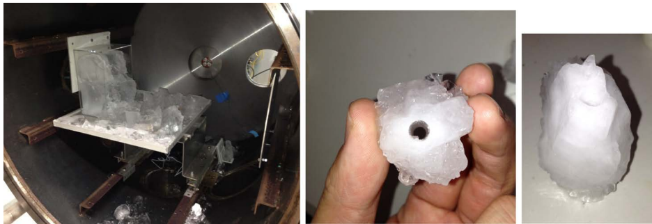
Figure 14. A block of recompressed fine-grained ice pieces and a trace of penetrator in it (left: Destroyed target, Middle: Recompressed ice piece (frontal view), Right: Recompressed ice piece (overall view).
