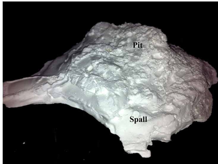
Figure 13. Surface roughness in pit and spall (note: The upper side of the picture corresponds to the bottom of the crater).
