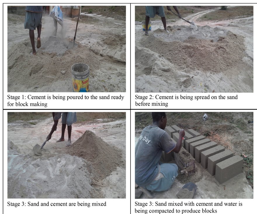
Figure 7. Local way of sand cement blocks manufacturing. Source: Photographed by T. Sakijege.
