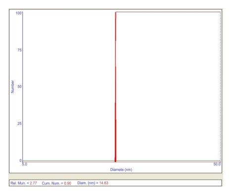
**Figure 2.** Size distribution of the TiO<sub>2</sub> nanoparticles determined by means of a Brookhaven plus 90 nanosizer.
