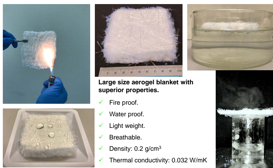
Figure 3. Large size aerogel blanket preparation.
