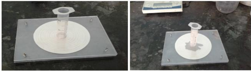
Plate 1. CST experimental setup (left) and CST experimental setup during filtration (right).
