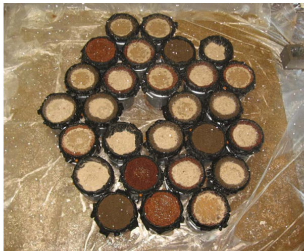
Figure 3. Actual layout of columns under rainfall simulator based on rainfall uniformity test.
