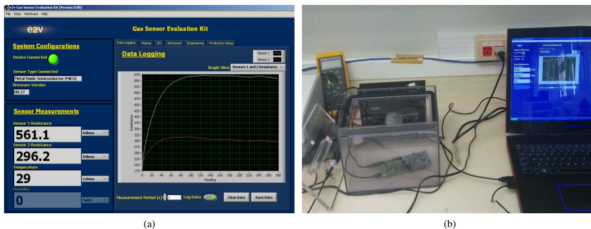
Figure 1. Kit MiCS-EK1 used to calibration the sensor. (a) Software Interface with readings of the slots; (b) Box of gas test (SR # 3) with the kit MiCS-EK1 connected to evaluation software.
