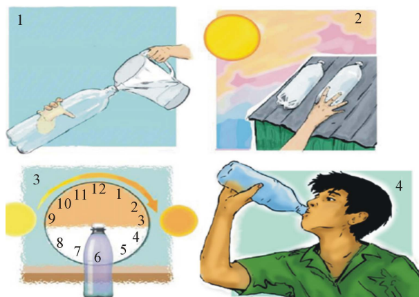
Figure 8. A graphical description on the solar disinfection (SODIS) household water treatment technique.
