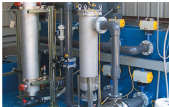
Figure 4. Membrane systems remove 0.05-micron particles from water.
