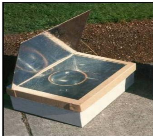
Figure 6. A solar pasteurization device in the shape of a box with a glass cover and a reflecting interior and folding lid. The water container is put inside the box and heated with solar heat. Source: CAWST [15].
