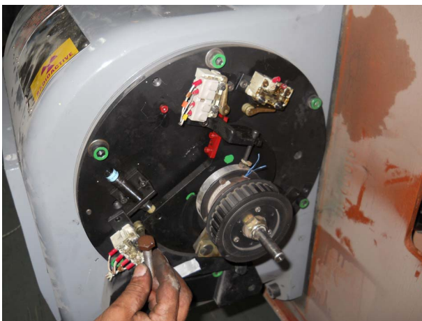
Figure 7. Insurance of safe position of radioactive source.
