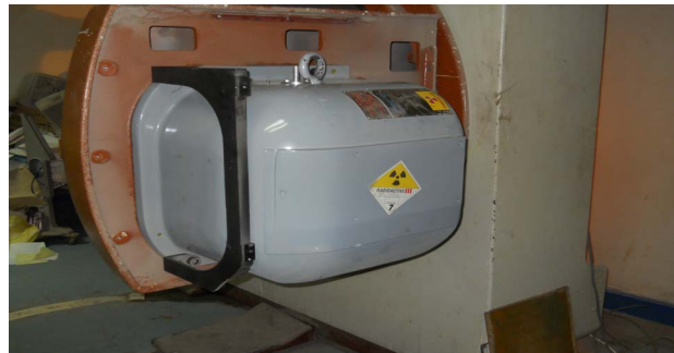
Figure 2. Head of ^{60}\text{Co} source; metallic support and its accessories.
