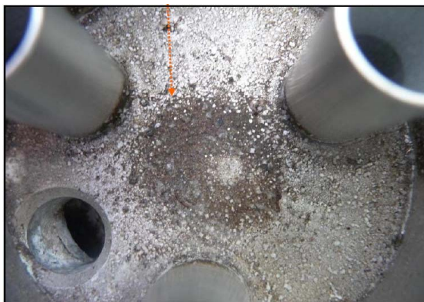
Figure 6. Photography showing the deposition of sea salt crystals inside the PM 10 sampling head at BON.
