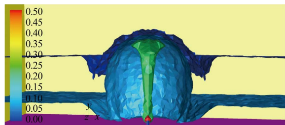
Figure 12. (penetration height = 0.292 m, Run No. 5), v = 0.5834 m/s, d = 0.1 m & density = 1.00736 \rho_w .
