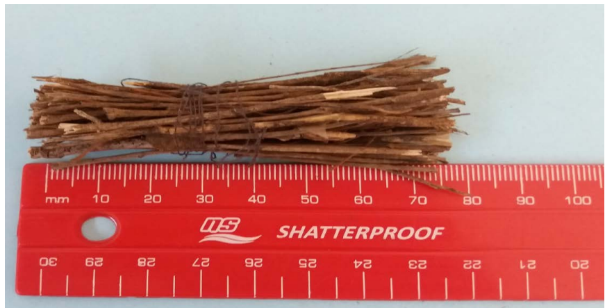
Figure 4. Combustion fuel (weeping wattle fine twigs) used for breakdown electric field measurement.
