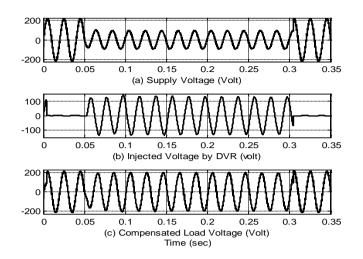
Figure 8. Behavior of system with DVR for nonlinear load by proposed controller.
