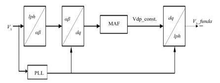
Figure 2. Fundamental positive sequence component extraction.
