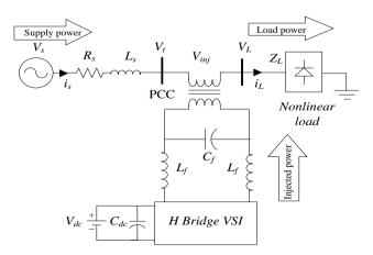
Figure 1. Single phase system configuration with DVR.
