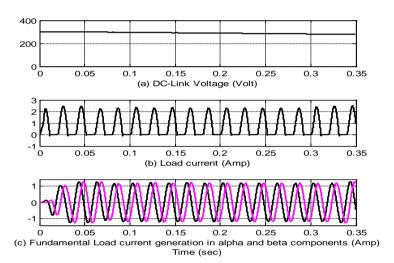
Figure 9. DC-link voltage and load current in case of nonlinear load.
