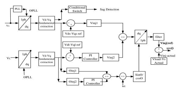
Figure 4. MATLAB based model of proposed control method.
