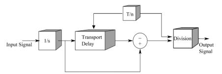
Figure 3. Block diagram of the moving average filter (MAF).
