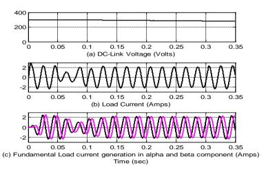
Figure 7. DC-link voltage and load current in case of linear load.
