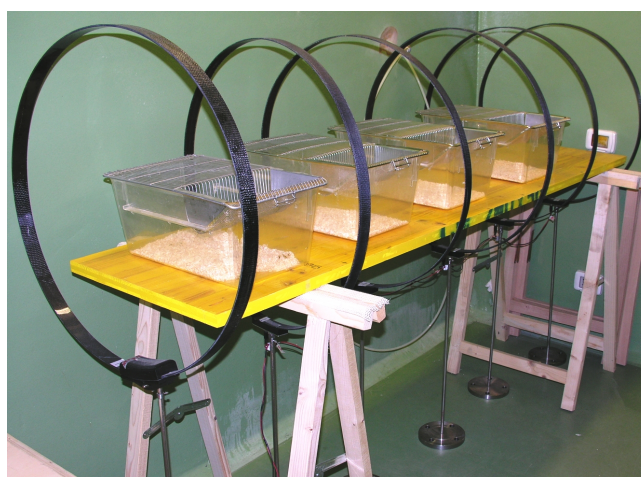
Figure 1. The exposure apparatus consisted of six coils in a Helmholtz configuration. Each coil, having a radius of 0.38 m, was made out of glass fibre, in which was embedded the copper wire. Coils are spaced 0.38 m, the total length of the exposure space was 1.9 m. Magnetic fields are generated by currents induced in the coils by a waveform generator.
