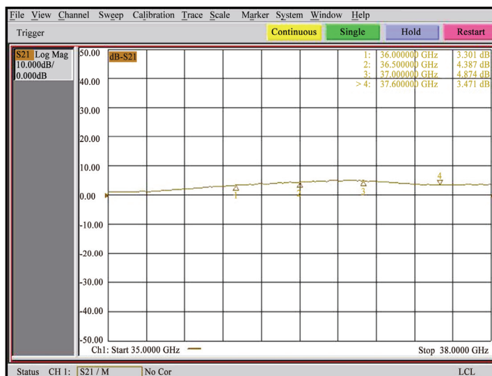
Figure 6. The gain of LNA after experiment
