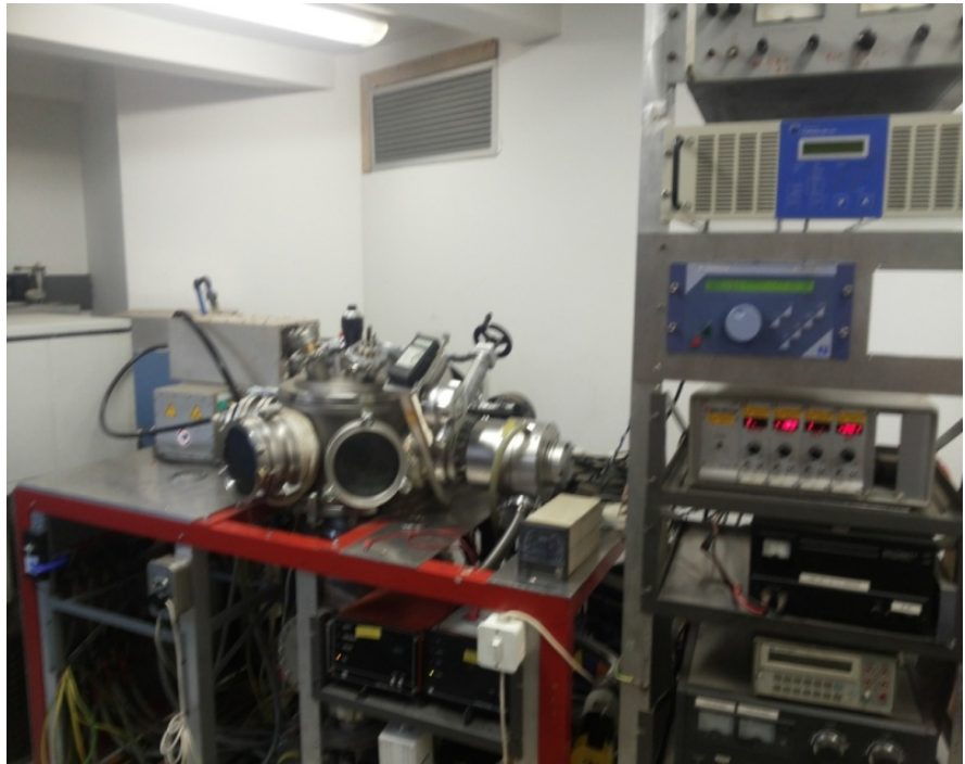
Figure 6. The sputter deposition system at laboratories of the faculty of science, University of Witwatersrand (Wits), South Africa.
