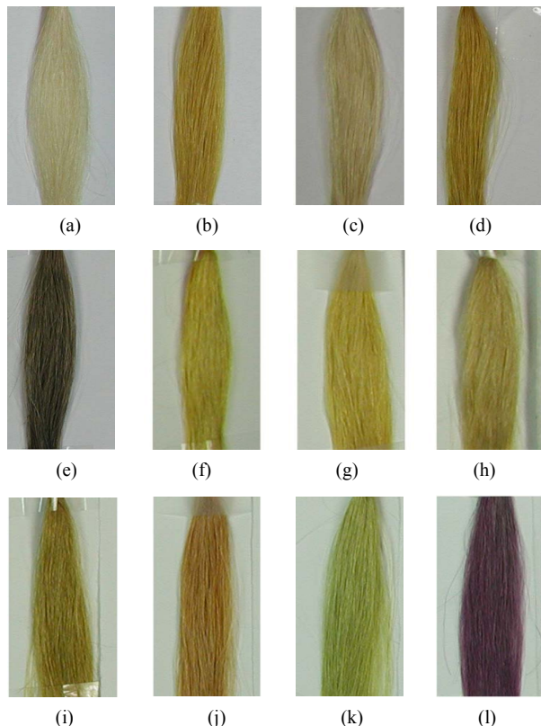
Figure 1. The photographs of undyed human hair (a) and the hair dyed by using tyrosinase with (+)-catechin (cat.) only (b), with cat. and L-cysteine (c), with cat. and L-tyrosine (d), with cat. and L-dopa (e), with cat. and naringenin (f), with cat. and lac (g), with cat. and tamarind (h), with cat. and hematoxylin (i), with cat. and kaoliang (j), with cat. and gardenia blue (k) and with cat. and red cabbage (l).
