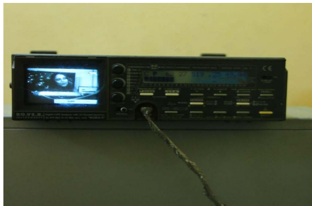
Figure 2. Field strength meter (CATV).
