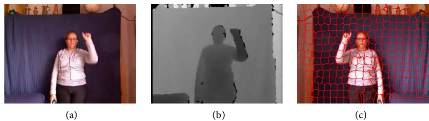
Figure 3. D_SP segmentation result. (a) RGB Image; (b) Depth Image; (c) D_SP Segmentation.
