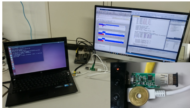
Current monitoring circuit
