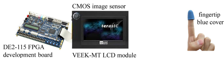
Figure 1. A fingertip writing character recognition system setup.
