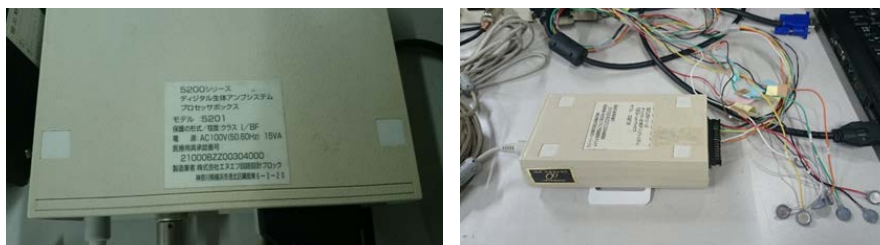
Figure 2. NF instrument processor box (Left picture) and EEG head box with electrodes (Right picture).
