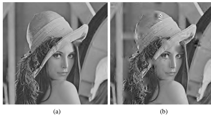
Figure 8. Image recovered by proposed scheme (a) compared with recovery by baseline system (b) at E_b/N_0 of 3 dB and D = 3 . PSNR of images (a) and (b) are 33.6 dB and 27 dB, respectively.
